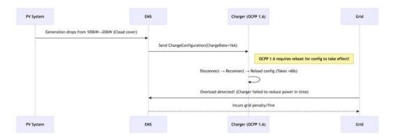
Since the configuration of OCPP 1.6 is device-level parameter modification, the configuration can only be effective after the charging pile restarts, and the real-time response of <300ms cannot be achieved.
