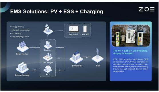
(5) Swedish Energy Storage Frequency Regulation Project: After receiving instructions from the VPP aggregator, the ZOE-EMS system can dispatch multiple PCS control signals to achieve 700 milliseconds FFR latency. This millisecond-level grid edge response capability enables the system to meet the requirements of the EU FCR market and generate verifiable ancillary service revenue through automatic bidding execution.
