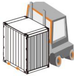
Figure 4.5 Forklift gear fully penetrates the forklift hole and protrudes
