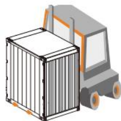
Figure 4.5 Forklift gear fully penetrates the forklift hole and protrudes
