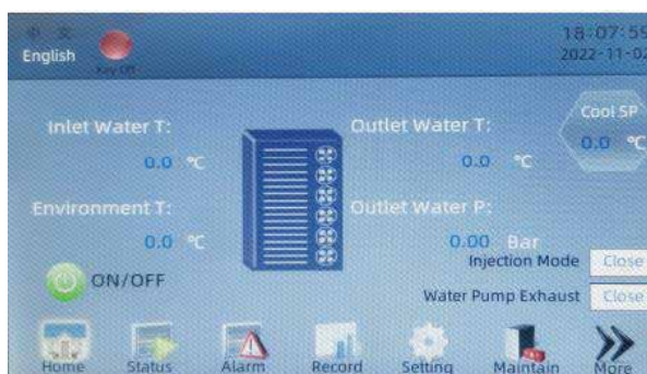
Figure 5-7: Control system homepage interface
