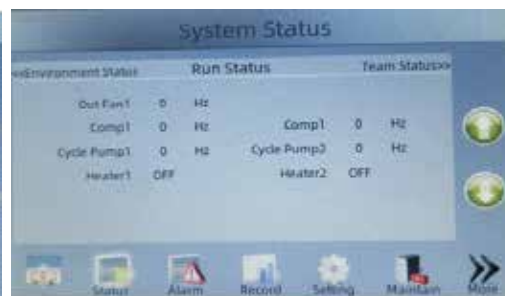
Figure 5-12: Run Status interface
