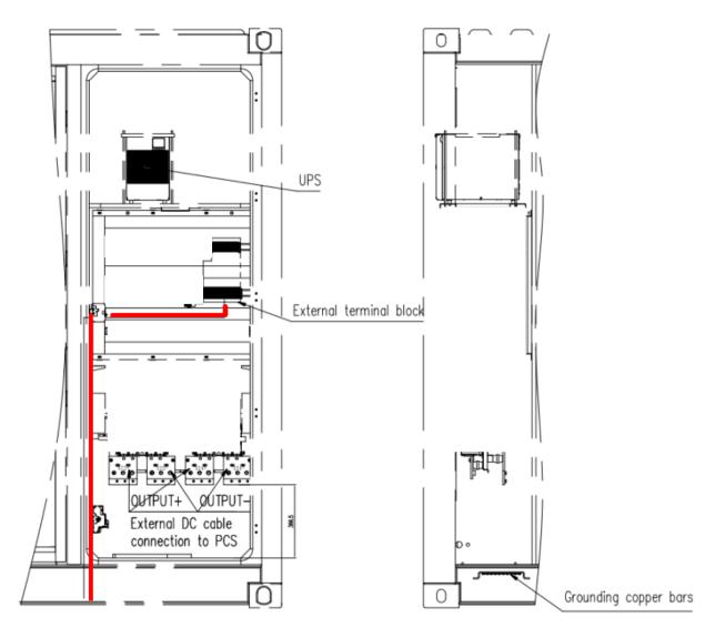
Fig.14 Schematic diagram of external cable connections in the electrical
