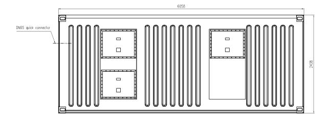
Fig.10 Water fire interface diagram
