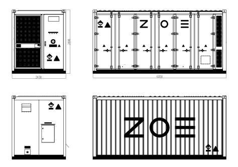
Fig.4 Appearance and Installation Dimensions
