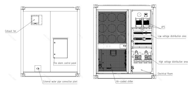
Fig.2 Layout of electrical room and fire suppression system
