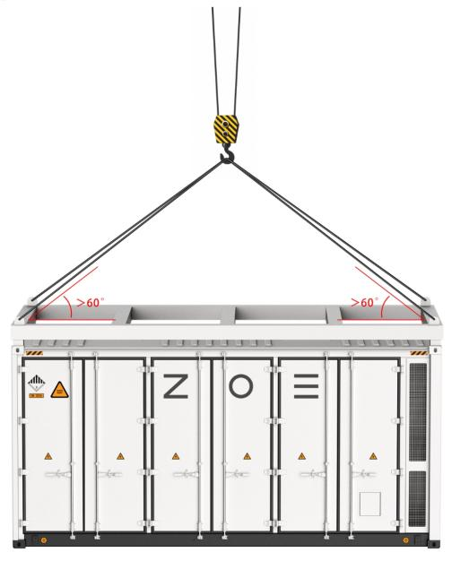
Fig.13 Hoisting diagram
