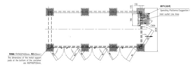
Fig.11 Mounting Hole Positions in Columns (Unit: mm)
