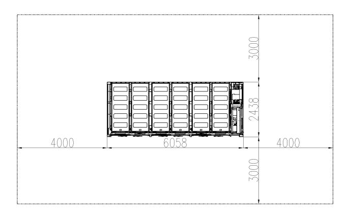
Fig.12 Schematic Diagram of Installation Space Requirements for a Single BESS (Unit: mm)
