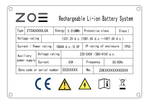
Fig.5 Nameplate Description Diagram
