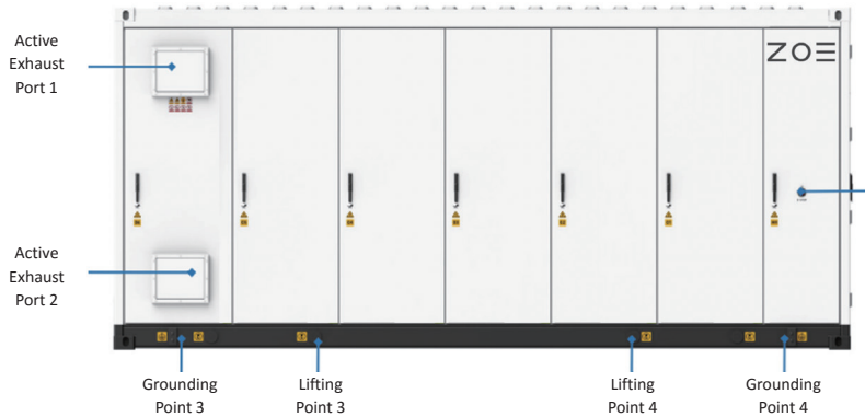
Figure 2-3 Rear View of Battery Container
